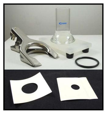
PortHoles Electrochemical Sample Masks define a known area of the sample surface for electrochemical testing with the PTCl. PortHoles are available in I, 3, or 10 cm<sup>2</sup> area to accommodate any specimen.
