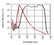
Figure 5 – Efficiency curve: 2400 g/mm. Red dashed curve: P-plane; solid black curve: S-plane.
