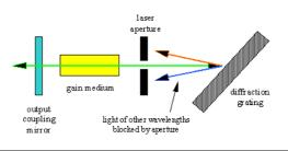
Figure 3 – Littman tuning using a grating near grazing incidence.
