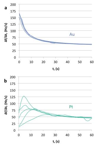
**Figure 2.** Rate change of frequency during the first 60 s of PEDOT(PSS) polymerization over Au (a) or Pt (b) electrodes on the surface of the quartz crystals<sup>4</sup>.
